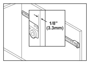
5. Using a level, ensure cabinet member (C) is level and secure to the wall using the provided screws.
