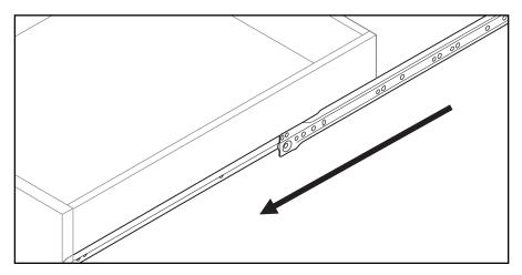
3. Once attached, measure the distance between the bottom of the drawer front to the top of the cabinet member (C) Write down this measurement "X".
